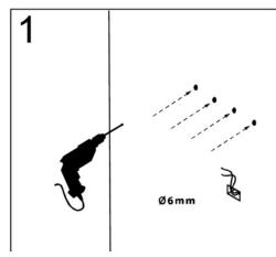
For drywall installation, mark the hole locations and drill  $\Phi$  6mm holes for the drywall anchors. Install a junction box behind the mirror for power connections.
